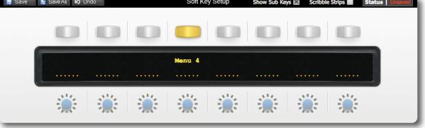
Clicking the **Show Sub Keys** box to the right of the **Soft Key Setup** label will blank the scribble strip shown in the Remote, leaving only those top row buttons which have been set to be menu selectors. The **Show Sub Keys** box will be checked (**X**) to
